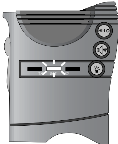
Fig 3.6 - 150 Battery Status LED
